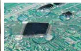
A silicone coated circuit board
